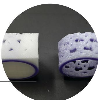
The MJP 300W Plus is the latest-generation 100% wax pattern 3D printer that adjusts to your workflow, delivering capability for both, several short run batches a day and overnight for larger builds. These highly accurate, fine wax patterns are directly printed, without the time, costs and geometric limitations of tooling.
