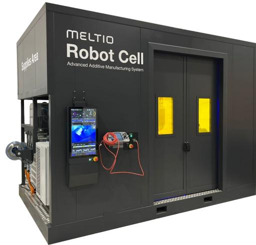
\* All these equipment and peripherals are anchored on this platform and may not exceed from the maximum dimensions of the self-supporting platform during transport.
